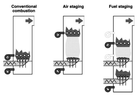
Figure. Principle of conventional two-stage combustion, air staging with reduction zone, and fuel staging with reduction zone.10
